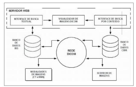
Figure 1. Architecture for a PACS-CBIR system.
