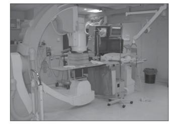
Figure 1. U-arc Philips H 3000 equipment utilized in interventional radiology with an image intensifier, two overhead monitors and patient table with controllers.
