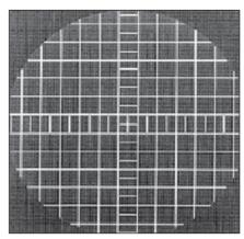
Figure 6. Image from a Leeds test object utilized to evaluate distortion on fluoroscopic equipment monitor screens<sup>(6)</sup>.
