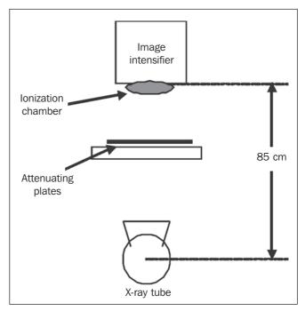
Figure 4. Positioning of ionization chamber and attenuating plates in relation to image intensifier and x-ray tube during measurement of image intensifier input air kerma rate.
