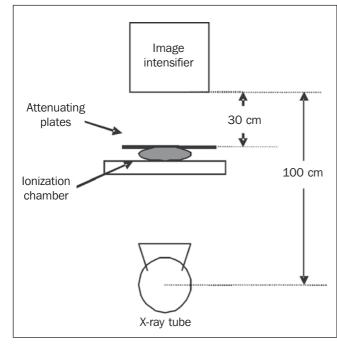
**Figure 3.** Positioning of an ionization chamber and attenuating plates in relation to images intensifier and x-ray tube during measurement of skin entrance air kerma rate.
