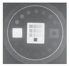
Figure 5. Image from a Leeds test object utilized to evaluate high- and low-contrast resolutions on fluoroscopic equipment monitor screens<sup>(6)</sup>.
