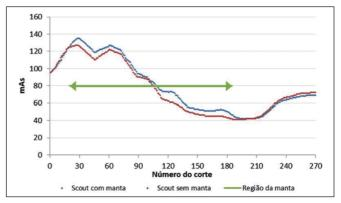
**Figure 3.** Comparison of the mAs profiles for scout with and without the presence of lead shielding.
