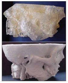
**Figure 5.** Prototypes constructed by the SLA (above) and SLS (below) processes based on a same tomographic data set. Note that the SLA prototype translucence makes the surface visualization difficult.
